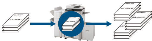
Multi-page original is scanned... stored in memory in proper page order... and stacked offset (or print data sent from PC)
