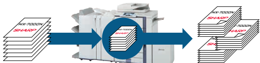
Multi-page original is scanned... stored on hard disk in proper page order... and stacked offset
